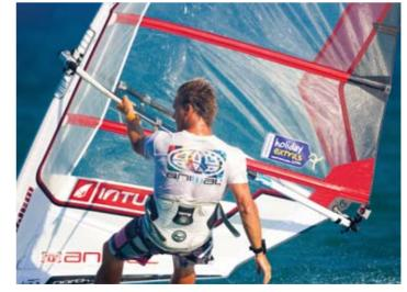
Batten tension- a massively overlooked feature of tuning- ensure all battens on the bottom third of your sail are cranked right on. On many camber induced sails, crank them on before you rig up, as once in the cams you can't get enough tension.
